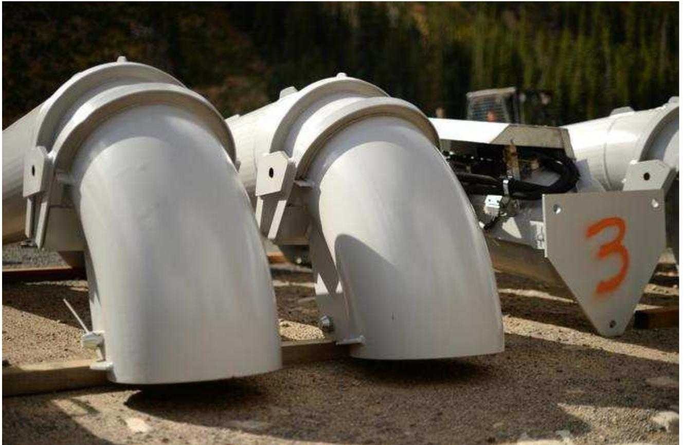
CDOT unveiled a Gazex avalanche mitigation system Friday that remotely uses compressed gases to create a concussive blast to trigger a slide. (*Hyoung Chang, The Denver Post*)
